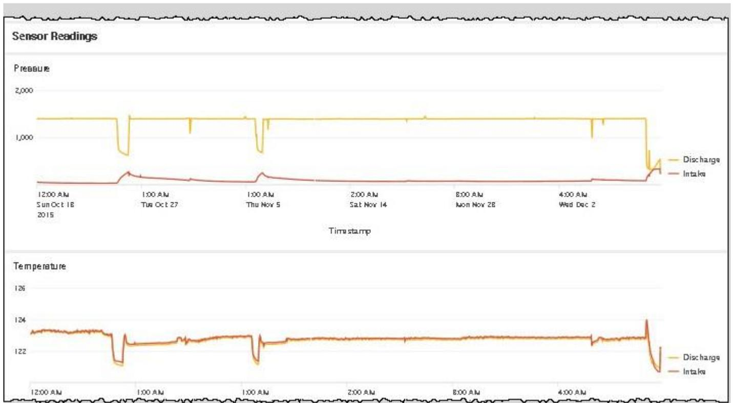
After a normal period, two significant alerts appear 45 and 33 days in advance of the failure.
