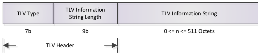
Figure A-11. Structure of an LLDP TLV
