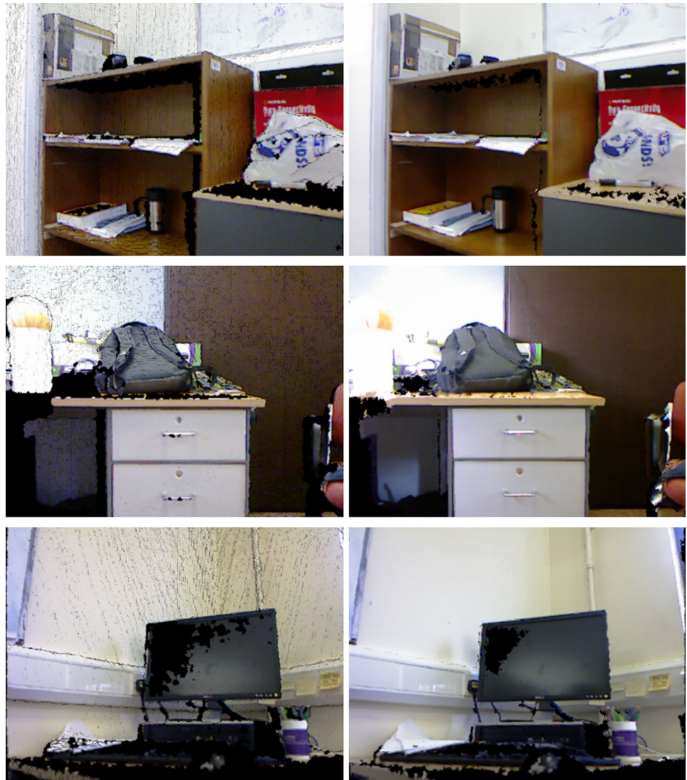
Fig. 8 On the left, raw 3D point clouds; and on the right, the corresponding filtered point clouds (Kalman filter)
