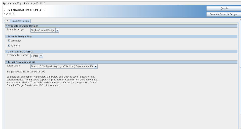
Figure 4. Example Design Tab in the 25G Ethernet Intel FPGA IP Parameter Editor
