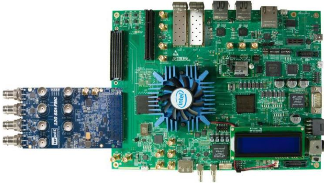
Figure 1-2. Inserting Terasic SDI-FMC Daughter Card into Development Kit Board FMC-A connector (J29).
