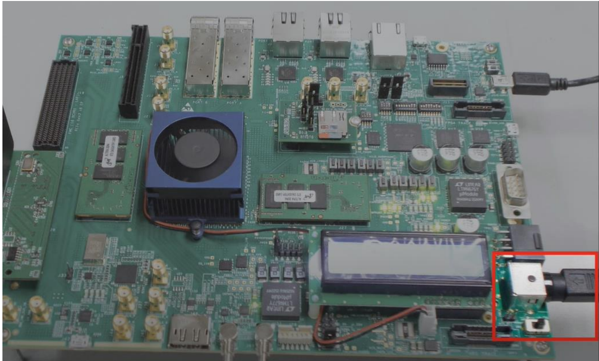
Figure 1-6. Connecting power supply to Development Kit Board DC_INPUT connector (J36) and powering on through the Power ON switch (SW5).
