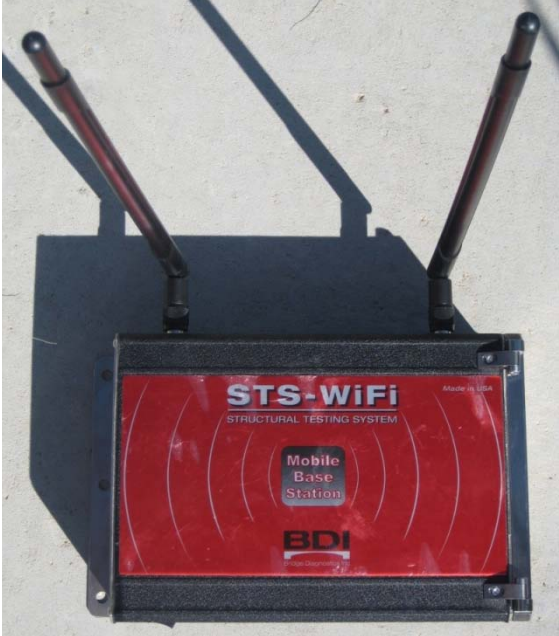
Figure 23. BDI mobile base station
