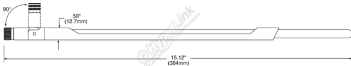
Figure 20. 9 dBi antenna (diagram courtesy of L-com)
