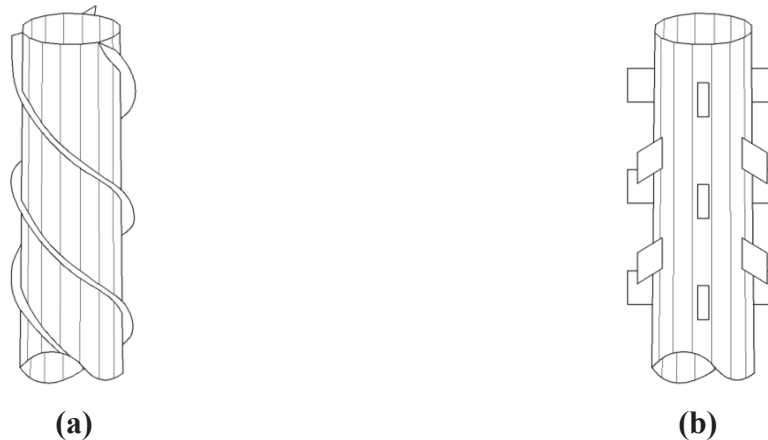
Figure 37. Add-on devices: (a) helical strakes (b) spoiler plates (after Kumar, Sohn, & Gowda, 2008)
