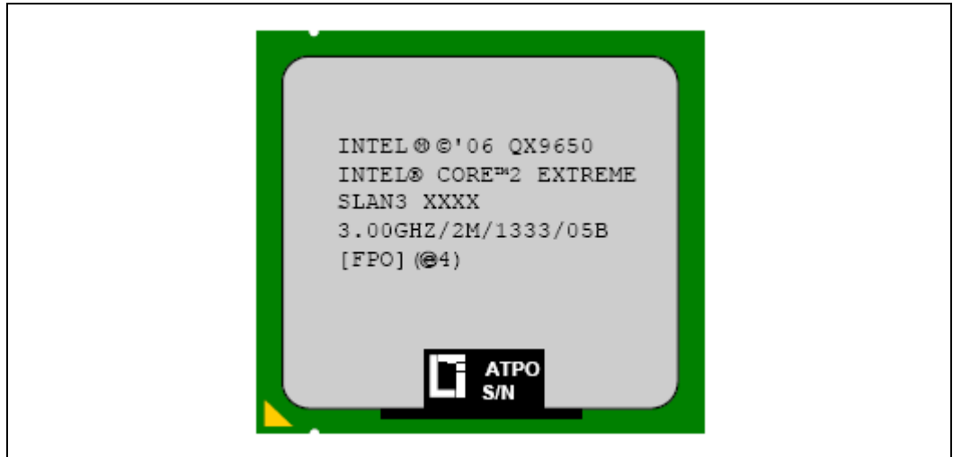
Figure 1. Processor Top-Side Markings Example (Intel® Core™2 Extreme Processor QX9650)
