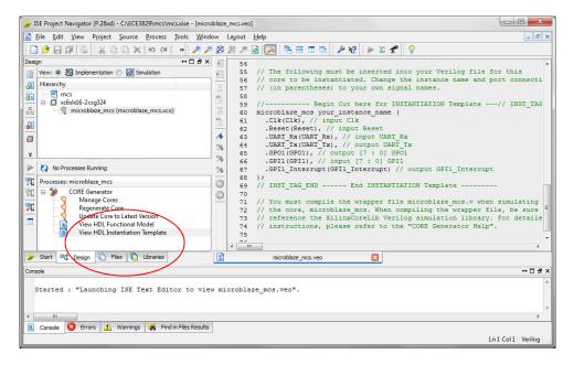
Create a new top level with connections to the clock and peripherals on the Nexys board and then instantiate the microblaze core by using the instantiation template provided.
