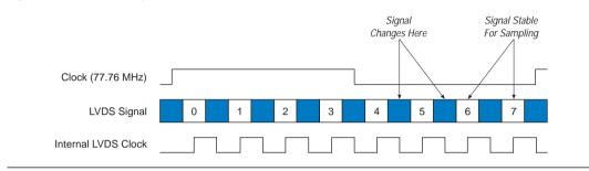
The 16 input LVDS channels in the input block, together with an LVDS PLL, clock the serial-to-parallel converter in the receiver. A parallel-toserial converter clocked by a separate PLL drives 16 output LVDS channels in the transmitter. The LVDS transmitter converts a maximum of 128 CMOS data bits on-chip into 16 LVDS data streams using an 8-to-1 parallel-to-serial converter. Similarly, the LVDS receiver converts the 16 LVDS data streams back into 128 CMOS data bits. See Figure 6.
