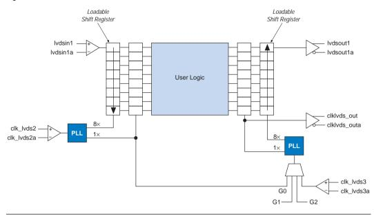
Figure 6. LVDS Receiver & Transmitter Interface
