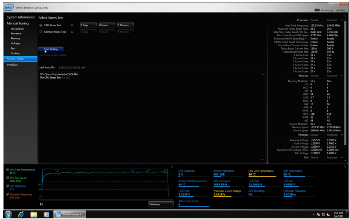
Figure 3.8. Intel Extreme Tuning Utility Showing Passing Stress Test Result on a Performance Tuned System Using an Intel Core i7-990X Processor and XMP 2133 MHz Memory
