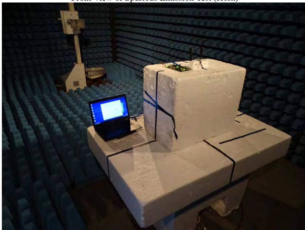
Front View of Spurious Emission Test (Horn)
