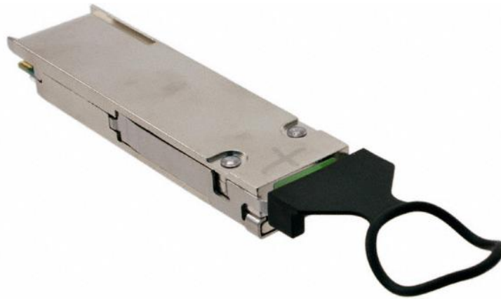
Figure 9-2 QSFP+ Loopback Fixture
