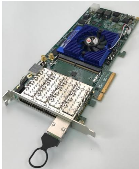
Figure 9-8 Setup QSPF loopback fixture
