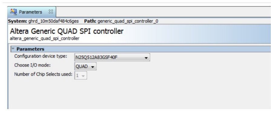
Figure 113. Generic Quad SPI Controller Parameter Settings
