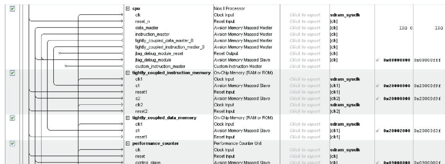
Figure 267. Connections for the Performance Counter
