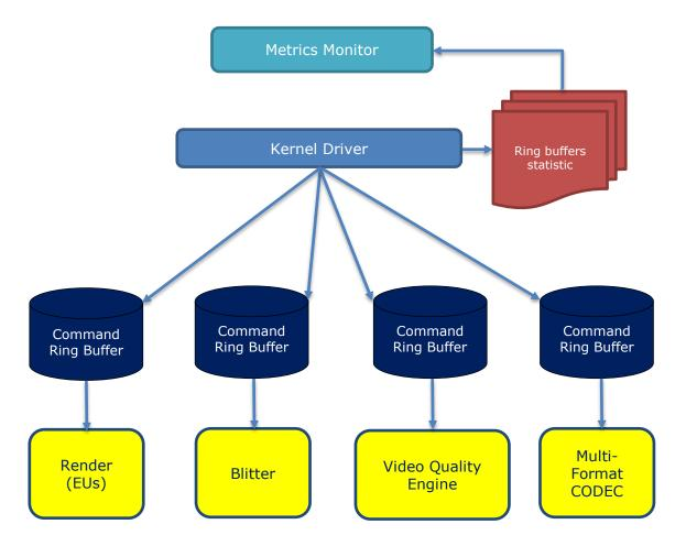
The usage of particular GPU unit is estimated according to the following data – "how much time the command ring buffer was in idle state during the sampling period".
